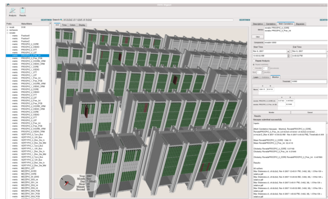
Fig. 2. Actual rendering of the Red Storm platform zoomed in on the partition on which data were taken. The nodes are colored red if below the user-defined probabilistic threshold for being too unreliable and green otherwise. Note that the metrics used in this example are the same two described by Figures 4 and 5. Grey indicates there was no data in the display time window for that resource for the metric being displayed.
