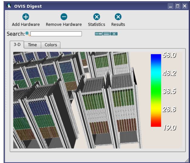
Figure 3. A screenshot of OVIS-2 with a physical view containing nodes colored by a metric value of a contained component (in this case, a microcontroller temperature) Note the strong dependence on height within the rack.
